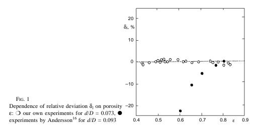
The experimental results by Andersson<sup>16</sup> for the next higher value of d/D measured by him are also given in Fig. 1. It can be seen that the absolute values of deviations are considerably higher as compared with the results of our own experiments for the value of ratio d/D = 0.073 and, beside that, they depend on the bed porosity, hence the approach suggested is no more satisfactory for the value of ratio d/D = 0.093.
